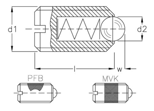
$\begin{array}{ll} \text{d1} & = \text{M10} \\ \text{d2} & = 6.0 \\ \text{Length I} & = 19 \\ \text{Spring pressure N bottom} = 45.0 \\ \text{Spring pressure N top} & = 24 \\ \text{W} & = 2.0 \\ \end{array}$
